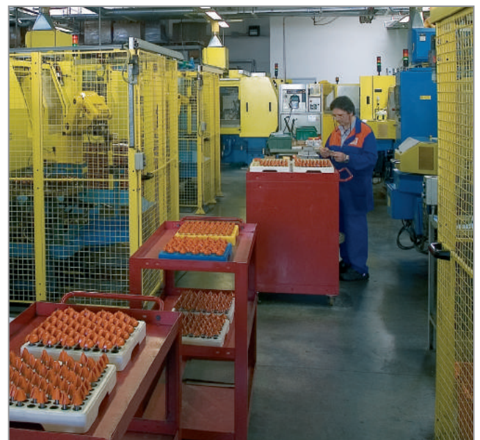
Loading the automated multi-axis CNC sharpening machines.
