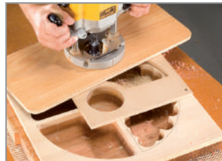
Rout the interior to final shape using the bowl and tray router bit and collet extension.
