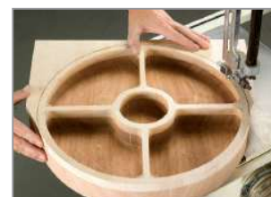
Bandsaw the exterior to final shape.
